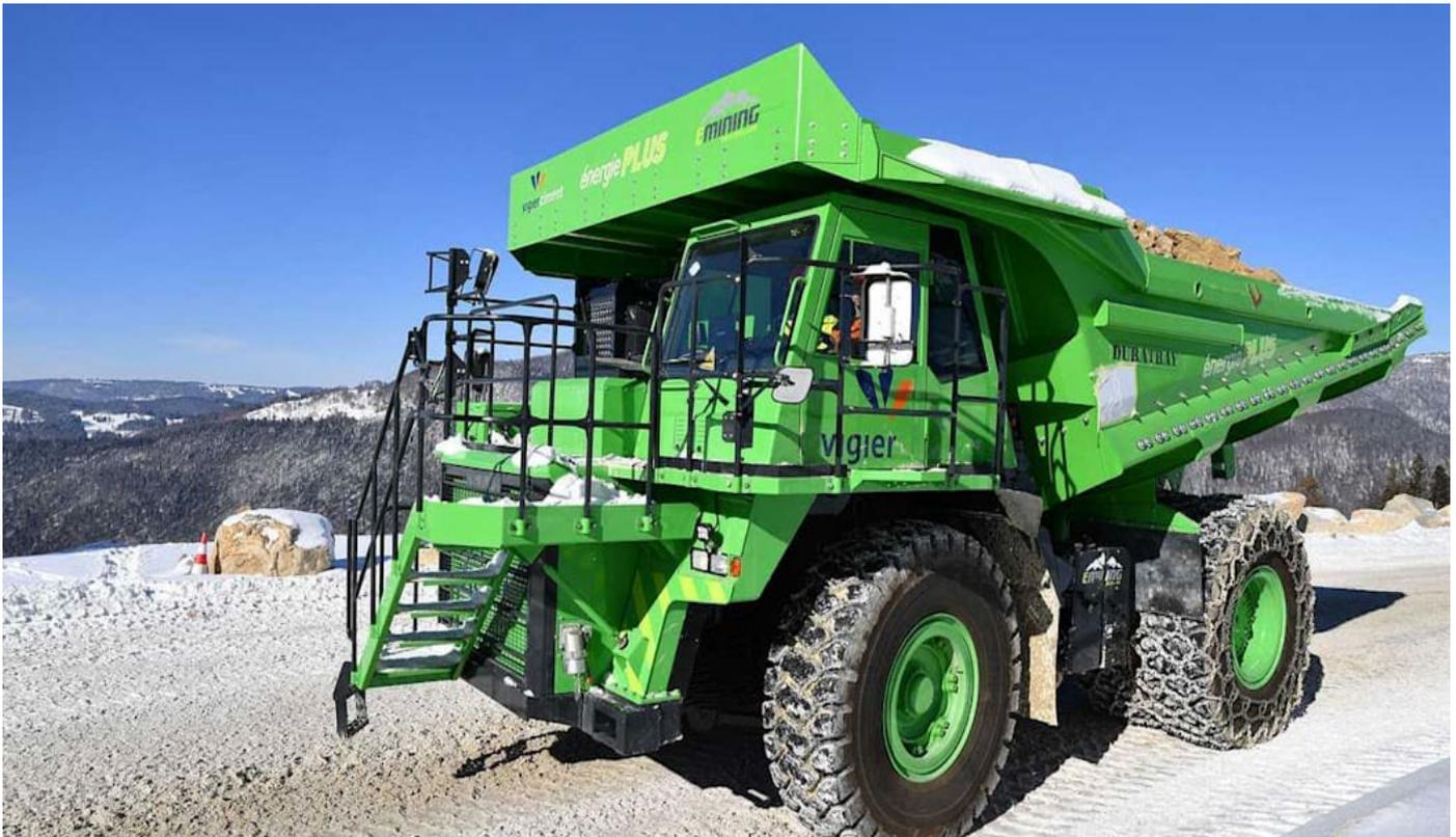
The Swiss division of machinery manufacturer Kuhn wants to electrify the mining **truck** segment. It converted a diesel-powered truck to run on electricity, and put the behemoth to work in a quarry located on the outskirts of Biel, Switzerland. Called eDumper, it's the largest **electric vehicle** in the world.
