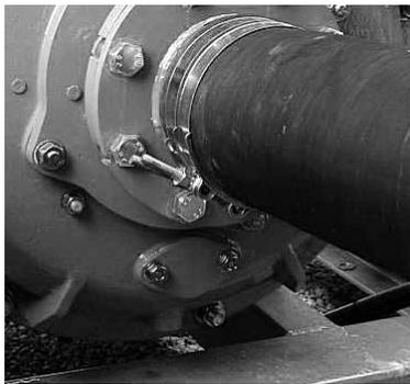
Pump drain for cold climate applications
