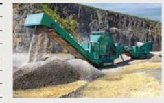
Engines are available that are certified to US EPA and EU off road diesel emission standards. Talk to your dealer about possible certification options (i.e. Tier 3/Stage 3A:, Tier 4l/Stage 3B:, Tier 4F / Stage 4).
